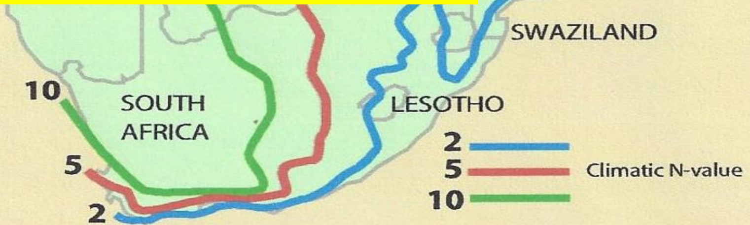
Figure 5.5 - Climatic N-value map of southern Africa 7 (currently does not cover the entire SADC region)
